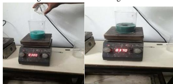
Fig Adding 8M \text{NaOH} solution dropwise, Color is changing bluish Green to black precipitate
