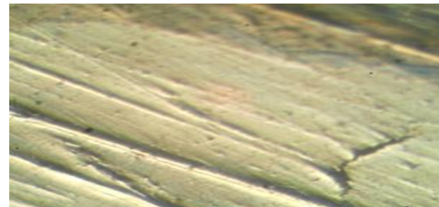
Fig 3.6 TIG welded AISI 316 L Weld metal Microstructure shows that Austenitic Structure in the welded zone.
