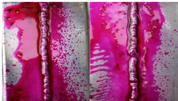
Fig 3.3 Liquid penetrant testing of Welded Plates of AISI 304 and AISI 316L
