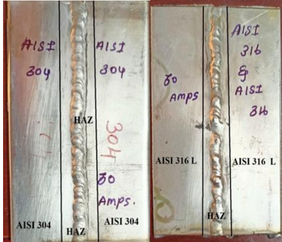
Fig 3.2 Visual inspection of Welded Plates of AISI 304 and AISI 316L
