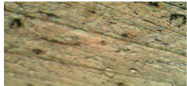
Fig 3.5 TIG welded AISI 304 HAZ Microstructure shows that grain coarsening observed at some areas on the heat affected zone.
