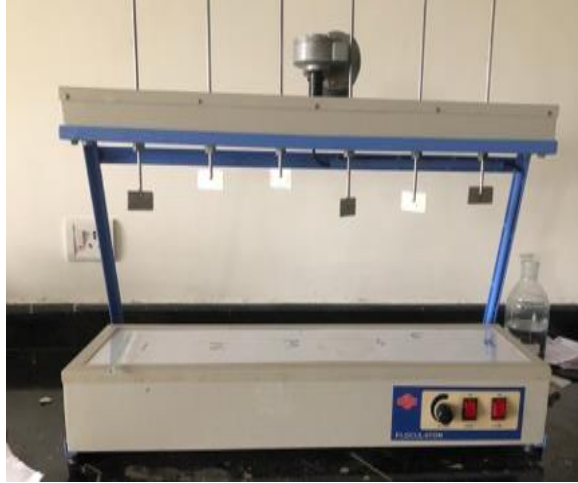
Figure3: Jar test apparatus setup
