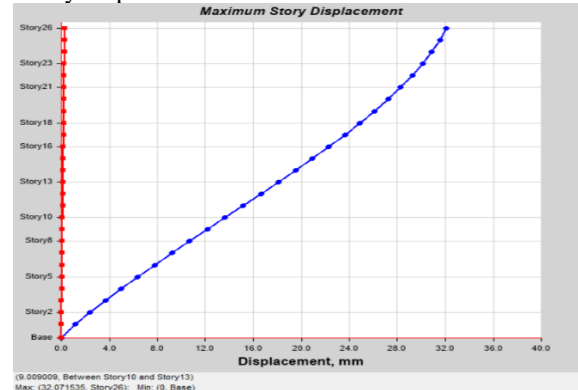
Figure 11: Max storey displacement for G+25 storeys building due to seismic forces
