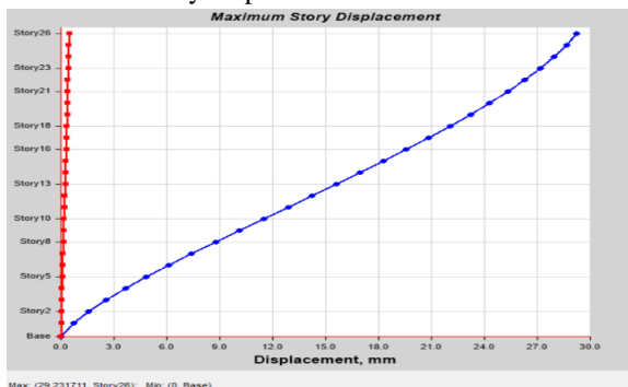
Figure 9: Max storey displacement for G+25 storeys building due to seismic forces
