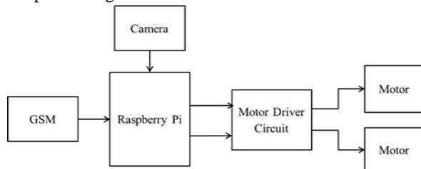
Fig 1 hardware module of proposed system
