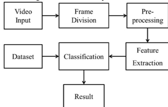
Fig 2 block diagram for image processing
