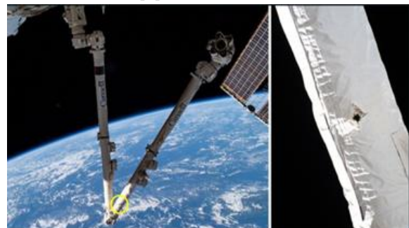
Fig.23: Hole in robotic arm caused by debris
