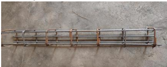
Figure 6. Steel reinforcement for Beam
