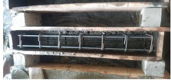
Figure 8. Steel reinforcement in Beam bonded with geosynthetics.
