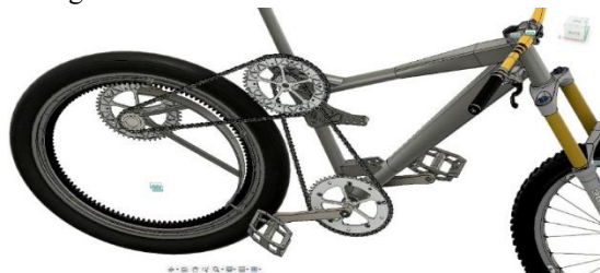
Fig: CAD MODEL "B" GEAR TRAIN MECHNISIM
