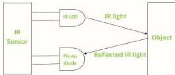
types of radiations are invisible to our eyes, but the infrared sensor can detect these radiations. When IR light falls on the photodiode, the resistances and the output voltages will change in proportion to the magnitude of the IR light received [5][6].
