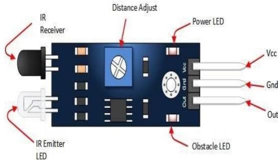
The infrared sensor is used to emits light to sense the object in the surroundings. It can measure the temperature of an object and detects the movement of things. Usually, in the infrared spectrum, all the objects radiate some form of thermal radiation. These
