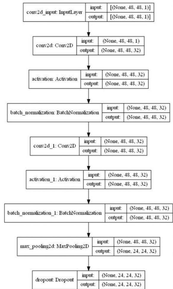
This is the flow of the first layer of the model. Here 32 is the number of filters that are eventually reduced when using max pooling. (3,3) is the size of the kernel. And the padding has been kept the “same” to protect the dimensionality of the volume. And the activation function used here was “elu”.
