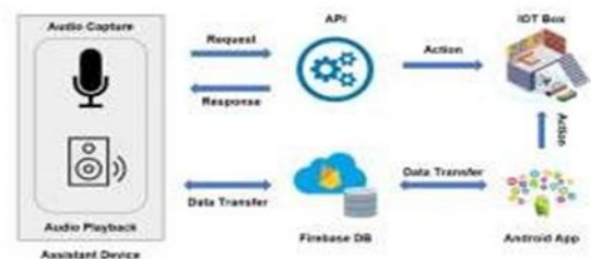
Fig 1. Basic architecture of Voice Controlled Personal Assistant
