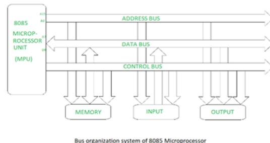
The system bus is a communication path between the microprocessor and peripherals. Mainly MPU
