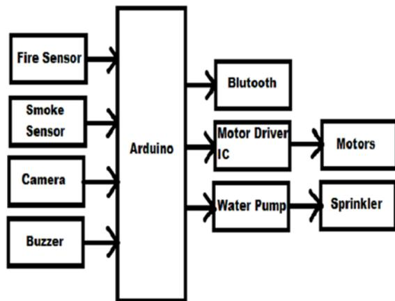
Figure 1:Block Diagram of Fire Extinguisher Robot
