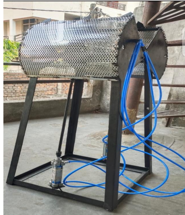
FIG.1. GALVANIZING TANK ZINC DIRT REMOVER”
