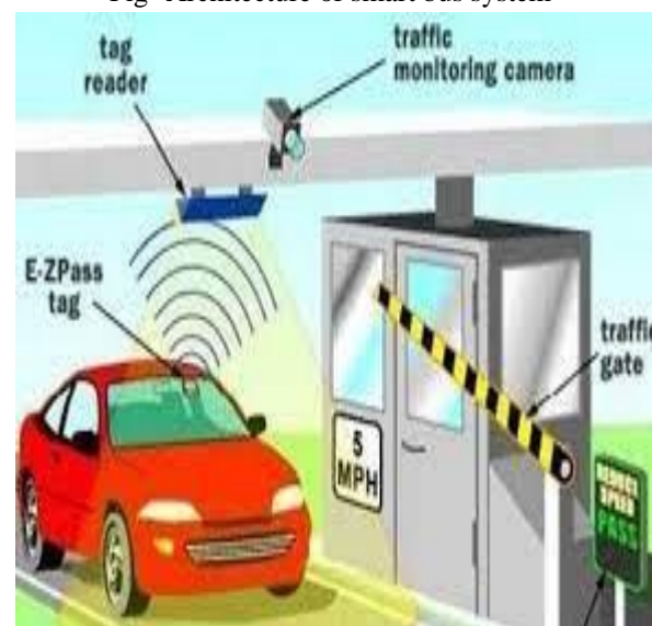
Fig- Architecture of smart toll booth system
