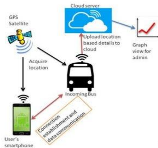
Fig- Architecture of smart bus system
