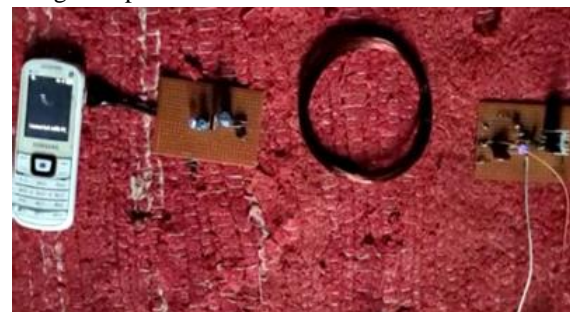
Fig. 13: Charging Phone using WPT
