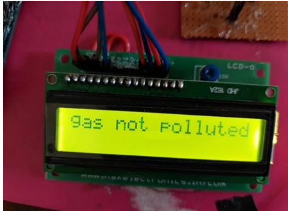
Fig 8: LCD display about Gas Polluted
