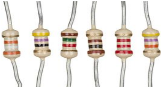
Fig. 6. Array of Axial Resistors - Color Coded to represent resistance
