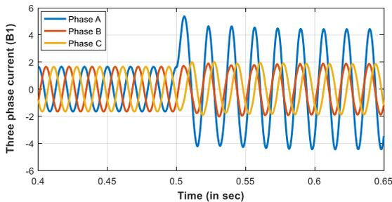
Fig 5.2 Three-phase current at Bus B1 (in pu) due to A-G fault during the grid-connected mode
