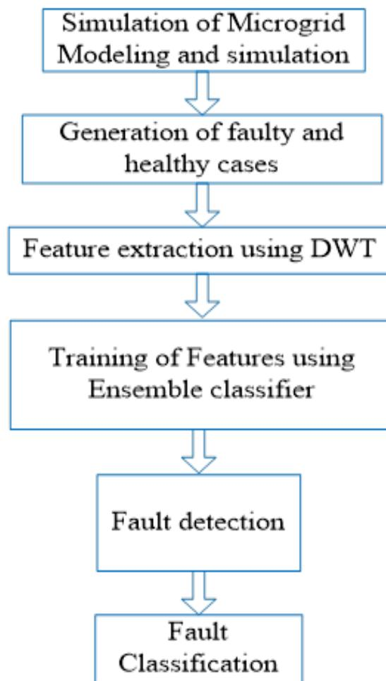
Fig. 2.2: Framework of proposed protection scheme
