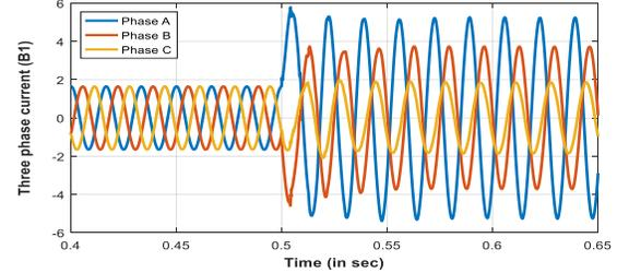
Fig 5.4: Three-phase current at Bus B1 (in pu) due to ABG fault during the Grid-connected Mode
