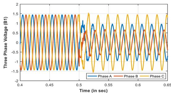
Fig 5.3 Three-phase Voltage at Bus B1 (in pu) due to ABG fault during the Grid-connected mode
