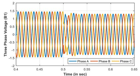
Fig. 5.5: Three-phase voltage at Bus B1 (in pu) due to ABCG fault during the islanded mode
