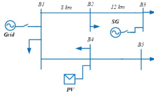
Fig.2 Microgrid system model
