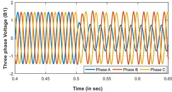
Fig. 5.1 Three-phase voltage at Bus B1 (in pu) due to A-G fault during the grid-connected mode.
