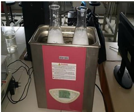
Fig. 1 : Ultrasonicator for preparation of nanofluid As for the Al 2 O 3 /water nanofluid, samples of 0.1% and 0.2% weight Aluminium oxide in base fluid (water) were prepared using ultrasonicator for about 8 hours. The nanoparticles were dispersed in water and ultrasonicated to obtain the solution of Al 2 O 3 /water nanofluid. The ultrasonication process prevents
