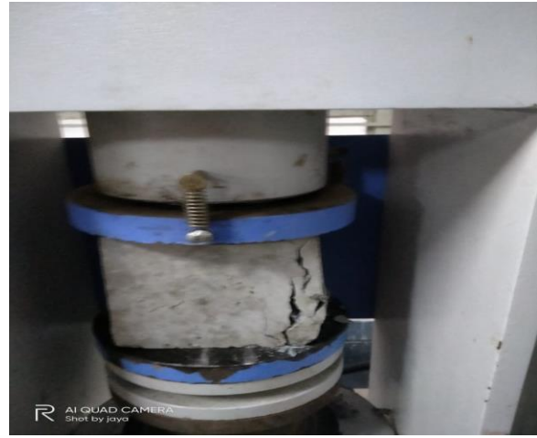
Figure: 3 Testing of concrete cube
