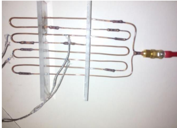
Figure 5: Third configuration (1.5mm and 2mm alternate internal diameter).
