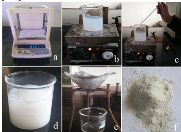
Figure 3: Experimental images of the synthesis process where (a) Weighing , (b) Stirring, (c)
