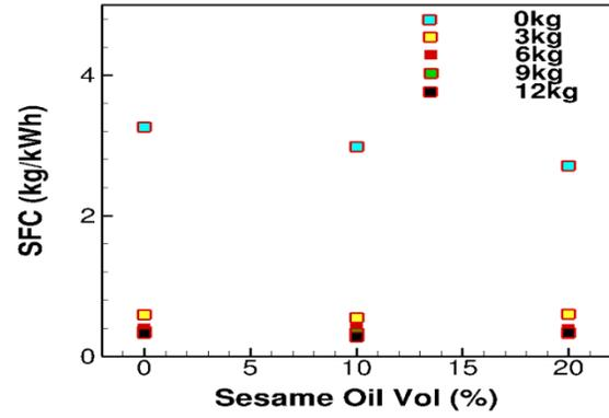
Figure 4 Variation of SFC with different types of bio-diesel
