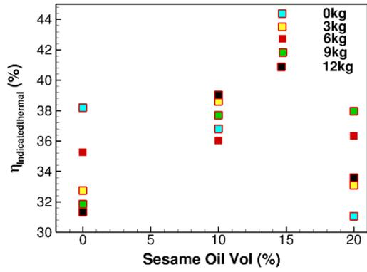
Figure 2 Variation of Indicated Thermal Efficiency with different types of bio-diesel
