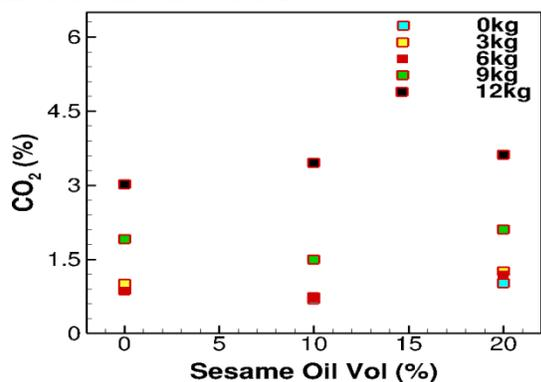
Figure 6 Variation of CO<sub>2</sub> emissions with different types of bio-diesel
