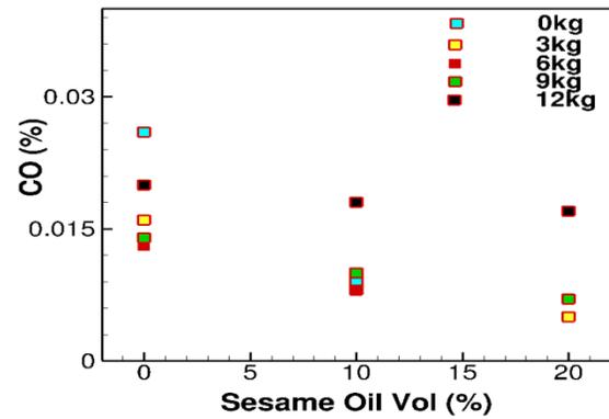
Figure 5 Variation of CO emissions with different types of bio-diesel
