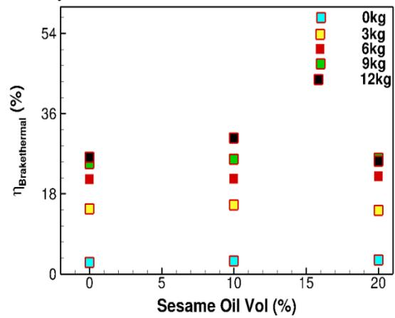
Figure 1 Variation of Brake Thermal Efficiency with different types of bio-diesel
