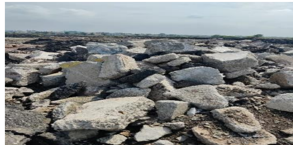
Figure 2 PQC Material Before crush
