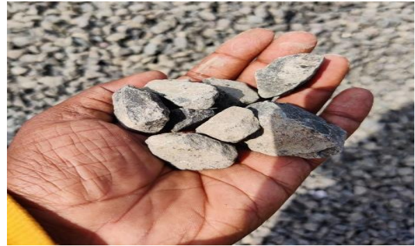
Figure 1 Granular sub-Base Material (GSB)
