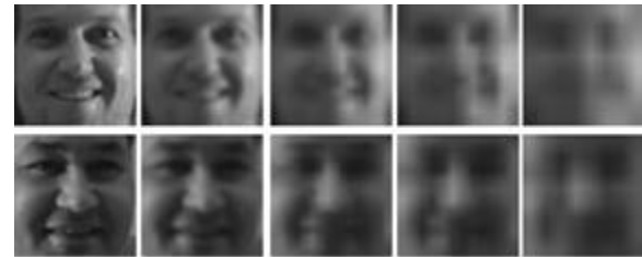
Fig 4: cropped face images high resolution to low resolution (left to right)
