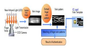
Step one: As shown in the device of our imaging device, the fingers provided for subject identification are exposed to a charge coupled device, also known as CCD, camera and an infrared camera, and we acquire input image. However, instead of using a CCD camera or a near-infrared camera, we use the information gathered from the database.
