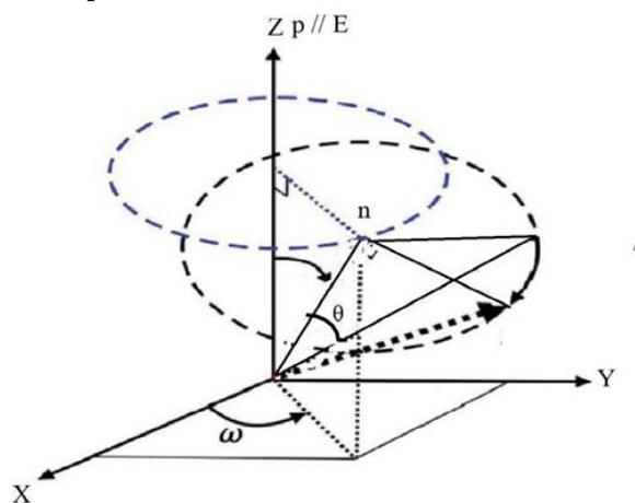
Figure 1. Illustration of the director with the cone angle between the director and the pitch axis under the external electric field
