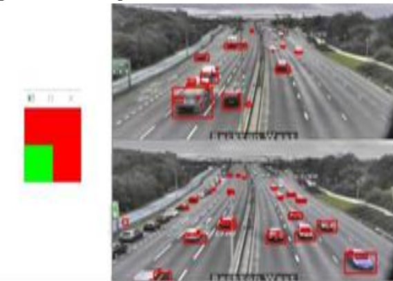
Fig. 5.Dynamic color change based on density The fig.5 shows the color change based on density. This is done using taking count of vehicles in each frame. If vehicle count of one of the quadrants is compared with other quadrants and also if it is a greater count than the others ,then green signal is indicated.
