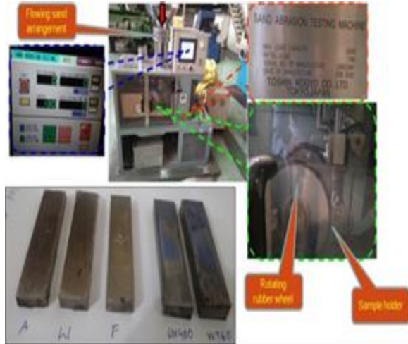
Figure 1. Dry sand- rubber wheel abrasion test machine, Toshin Kogaya.
