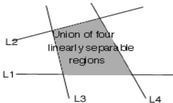
Figure3.3 Intersection of 4 linearly separable regions forms the center region.
