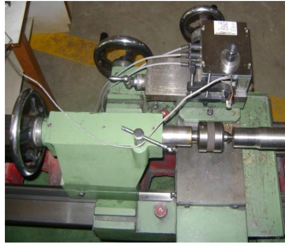
Fig 1 shows the arrangement made to measure the cutting temperature.
