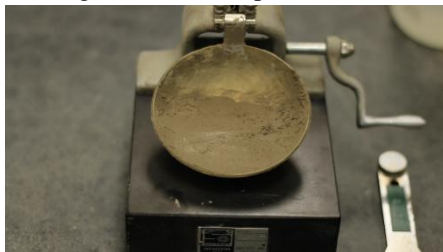
Fig. No. 2.2 Cassagrande's Liquid Limit Device
