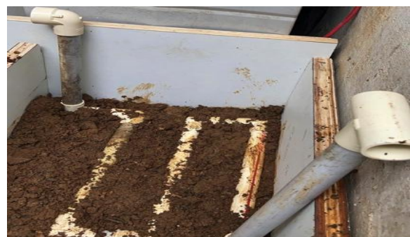
Fig. 7 Installing PVC pipes for EAT in the model
