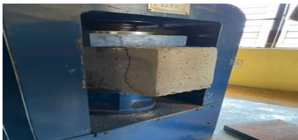
Fig. 4 Compression test for FAL-G block
