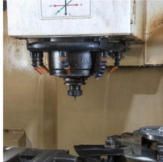
Fig. 2: VMC with vertically oriented spindle
