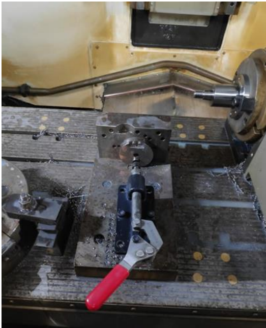
Fig. 7. Complete Assembly of Toggle Clamp with Fixture Bed
