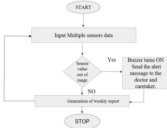
Fig 4.2: Block diagram for Health-Monitoring System
