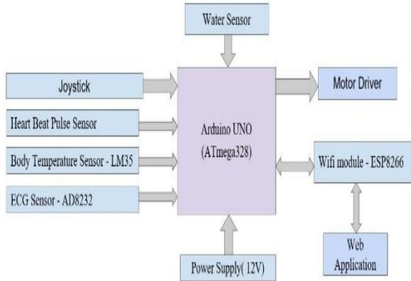
Fig 4.1: Overall functioning with respect to Arduino UNO
