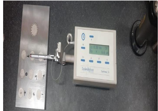
Figure.2.Pictorial view of portable surface tester
