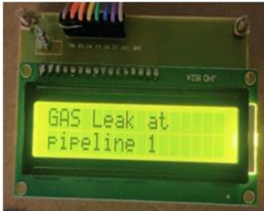
Fig 8: Display of LCD when leakage occurs
