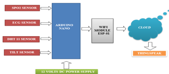
Fig1: Block diagram of health monitoring system
