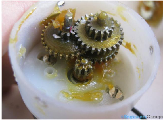
Figure.2. Shape of Bottom Gear Assembly
