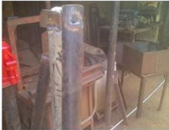
Plate 1. Drilled Hole on one end of the crane's arm
