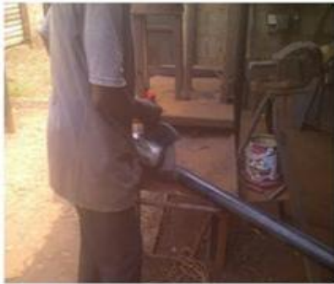
Plate 2. Grinding of the ram rest on the arm
