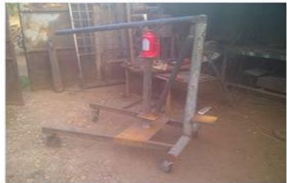
Plate 5. Crane assembly with hydraulic jack fixed
