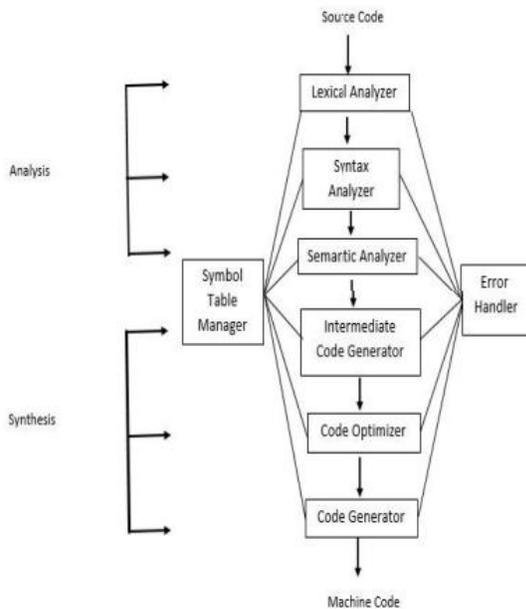
Fig 2: Block Diagram of Compiler
