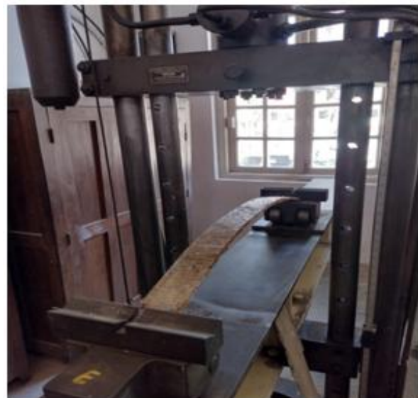
Fig.1. Bamboo e-glass fiber composite leaf spring undergoing a Max. deflection test on a leaf spring testing machine.
