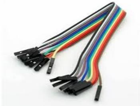
Figure E: Jumper wires
