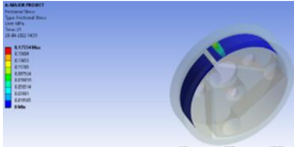
Figure 21 Frictional stress generated on the clutch plate(0.175Mpa)
