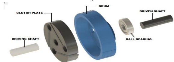
Figure 1 Parts of compliant centrifugal clutch
