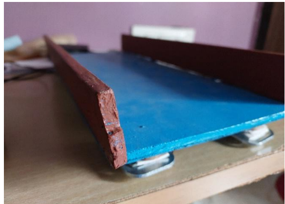
Fig. 7 Bridge With Load Cells on Pier
