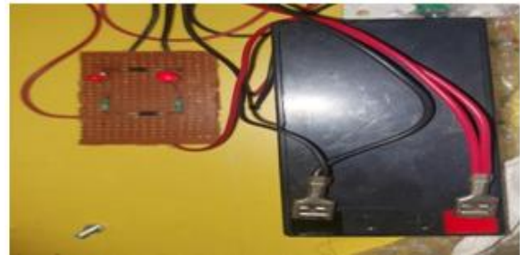
Fig.3 reverse protection circuit
