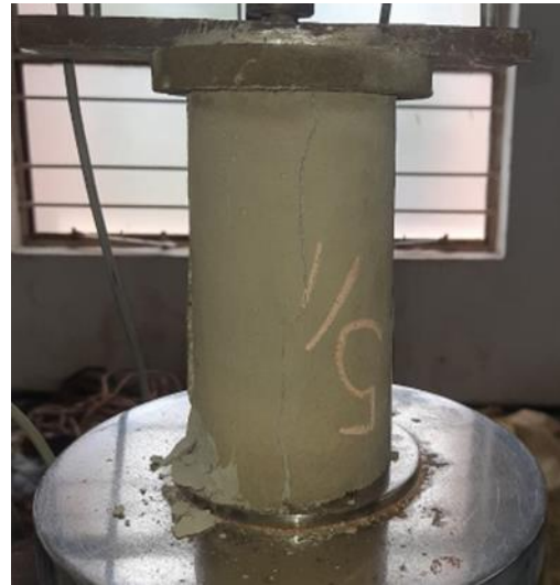
Fig.5.4: Failure pattern of fly ash-based material specimen
