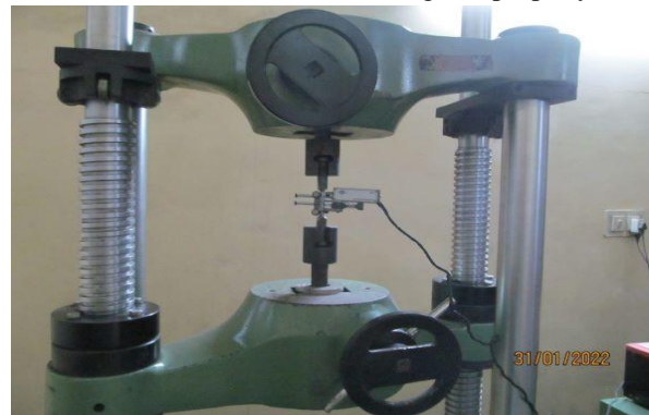
Fig-4.3: Tensile Testing by UTM
