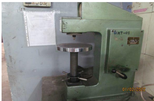
Fig-4.2: Rockwell/Brinell Hardness Tester.
