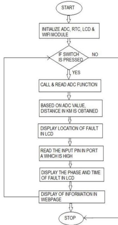
Flow Chart of Fault Detection System
