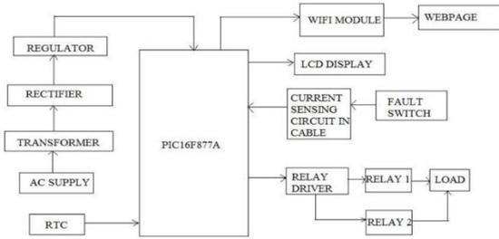
BLOCK DIAGRAM OF FAULT DETECTION SYSTEM
